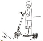
Do not ride at high speed when you get over speed bumps, thresholds etc., please ride at low speed on rough roads.
