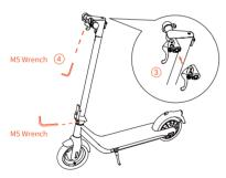
3. Place the brake lever on the handlebar, tighten it firmly with hex wrench to be sure it won't loosen. (Note: Use the M5 wrench to re-tight the folding part's nuts in case it's loosen after long time use)
